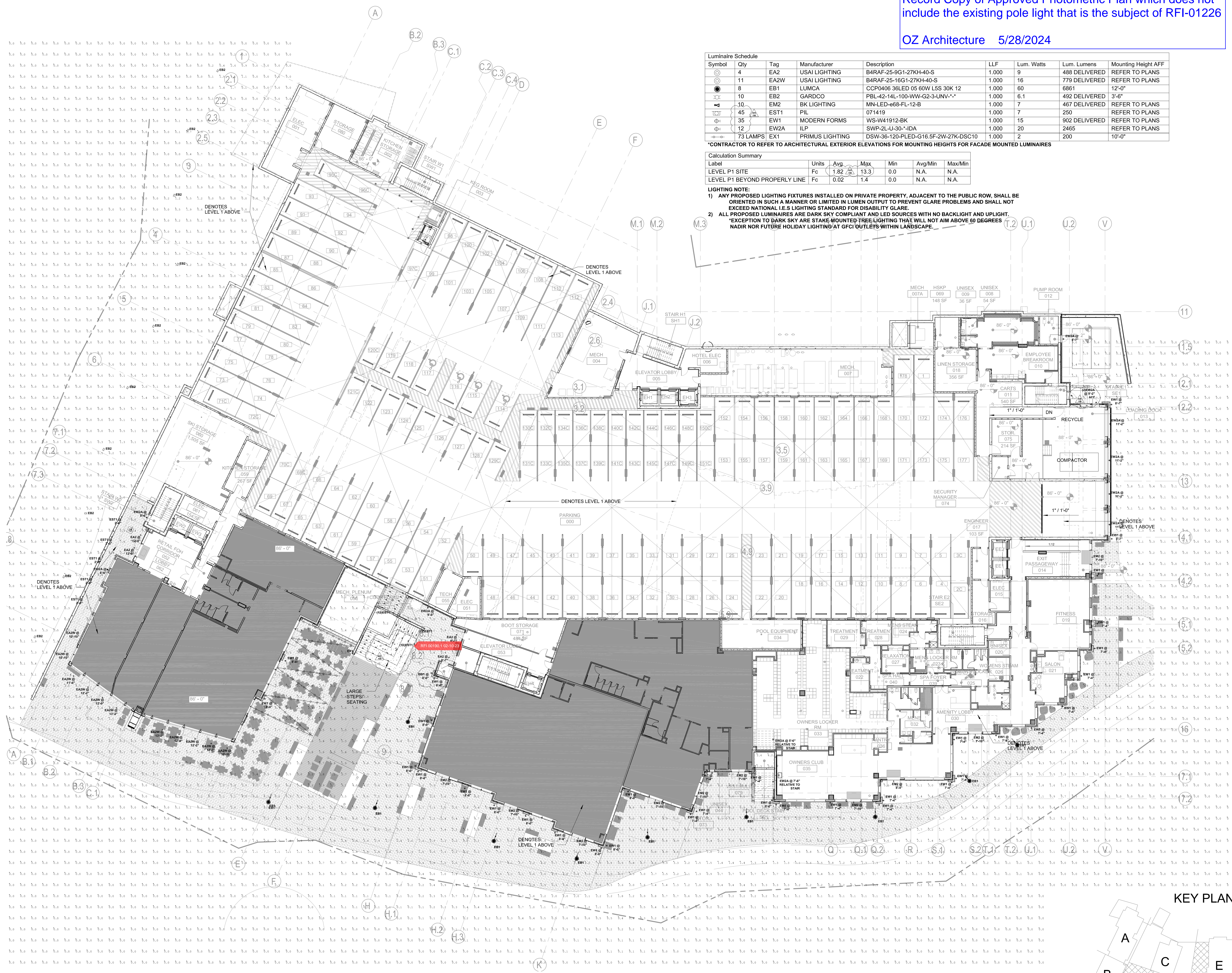
1 PARKING GARAGE SITE PHOTOMETRIC PLAN - OVERALL 1/16" = 1'-0"
