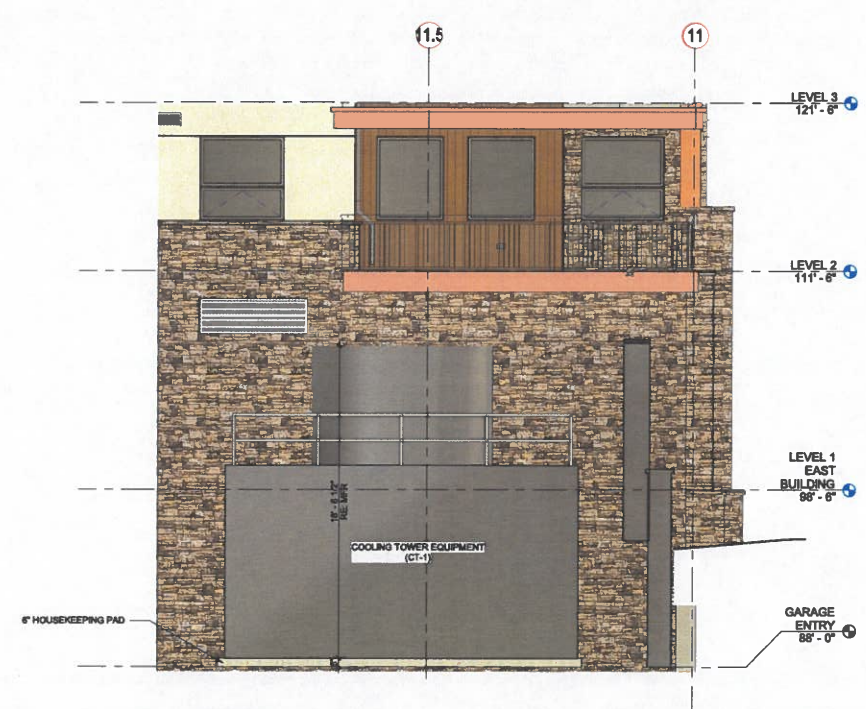
ENLARGED EAST SECTION - COOLING TOWER
